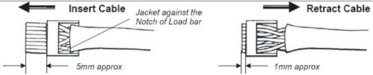
Figure 12: Insert Wires into Load Bar and Trim
