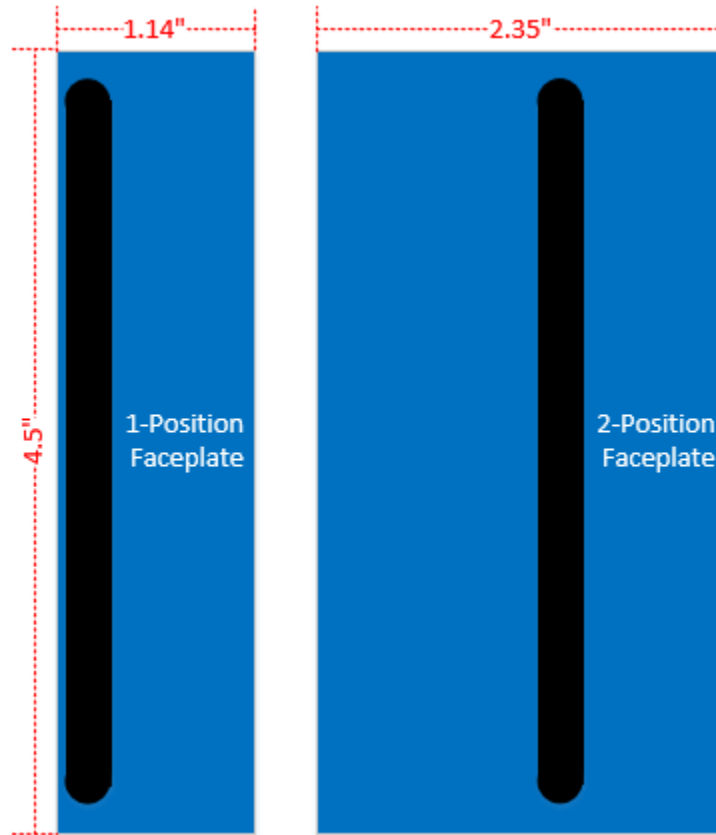
Figure 14: TCIB-UNI Faceplate Dimensions
