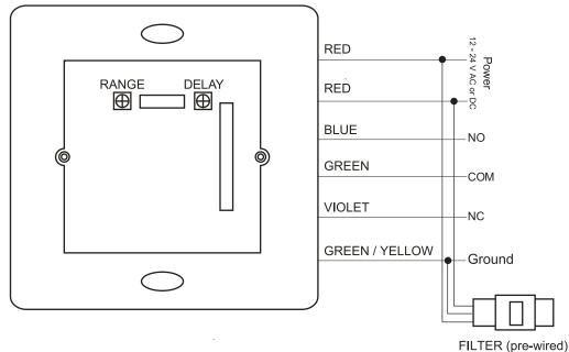
Typical wiring: Red wires connect to 12 - 24 V AC or DC.
