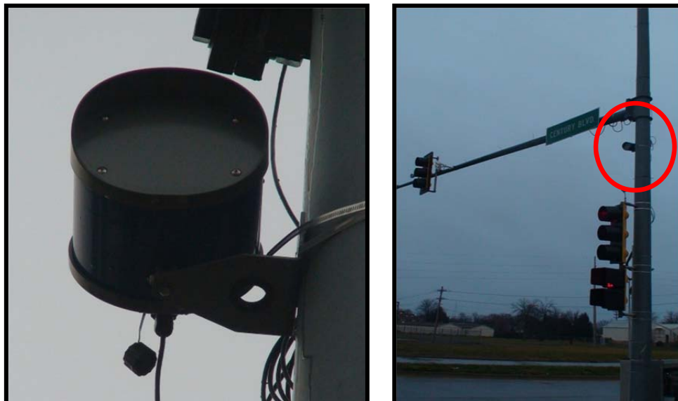
Figure 2. Sample pictures of the Intersector unit facing eastbound traffic.
