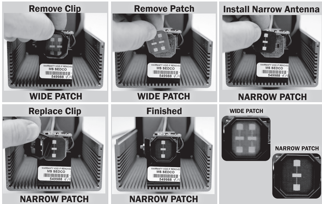
FIGURE 1b Switching from Wide* to Narrow Patch Antenna
