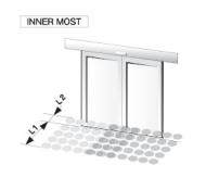
(These detection patterns are approximate and will vary slightly. Walk-test the unit to assure the pattern desired.)
