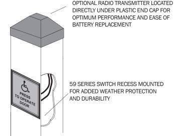
**59 SERIES SWITCH RECESS MOUNTED** FOR ADDED WEATHER PROTECTION AND DURABILITY
