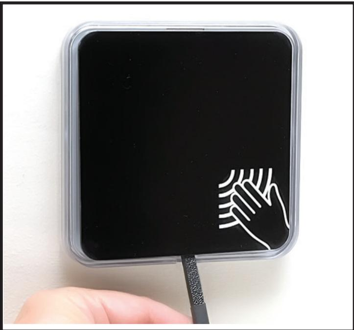
1. Remove faceplate using a screwdriver as shown.
