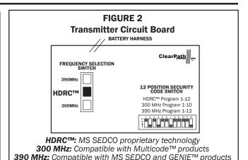
4) Insert the coin cell battery (provided) with the plus (+) side facing up (visible when inserted).
